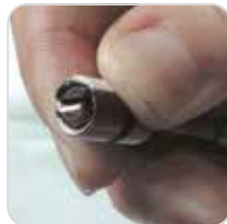
3. Load coiled insert into applicator
